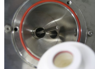
Fig. 7: Replacing filter: Inserting the new exhaust filter cartridge
